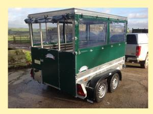
With the top removed the base unit can be used to transport a variety of goods. The trailer has side rope hooks and fitting points for extra fit options including: ladder rack, mesh sides, extended tailgate and livestock (sheep/pig) top with ramp.
